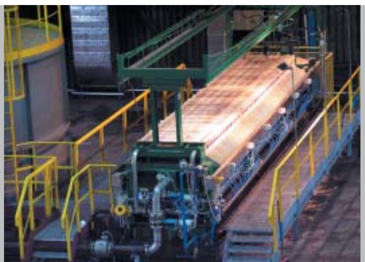
Filter press with PVDF membrane- and combination chamber plate 1200 x 1200 mm, application Metallurgy, chemistry etc.
