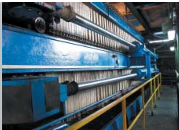
SALA filter press with JVK membrane- and combination chamber plates 1500 x 1500 mm
