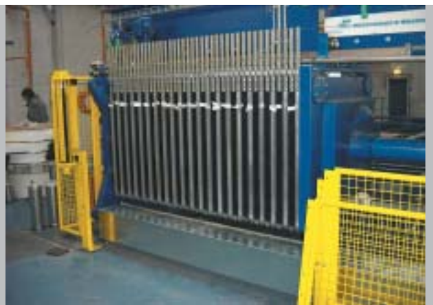
Filter press with membrane- and combination chamber plates 1200 x 1200 mm. Filtration of metal pigments with solvents, 16 bar squeezing pressure
