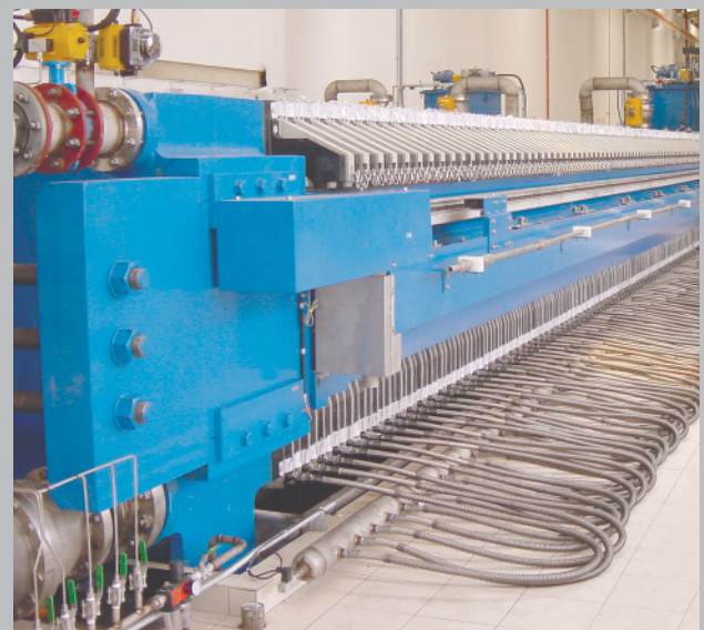
filter press with high performance membrane chamber plates 1500 x 1500 mm up to 5,0 MPa (50 bar)
